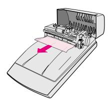
4 If you still cannot remove the paper from the ADF, lift the ADF lid to its fully open position, loosen the jammed paper from the roller at the rear of of the ADF lid, pull it gently from the ADF.
